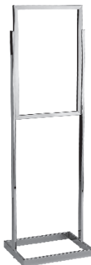
# BURT28 22"X28" SIGN HOLDER Vertical frame and base are made of rectangular tubing 1/2"X1 1/2". Base 15"X23 1/2". Height 56"
